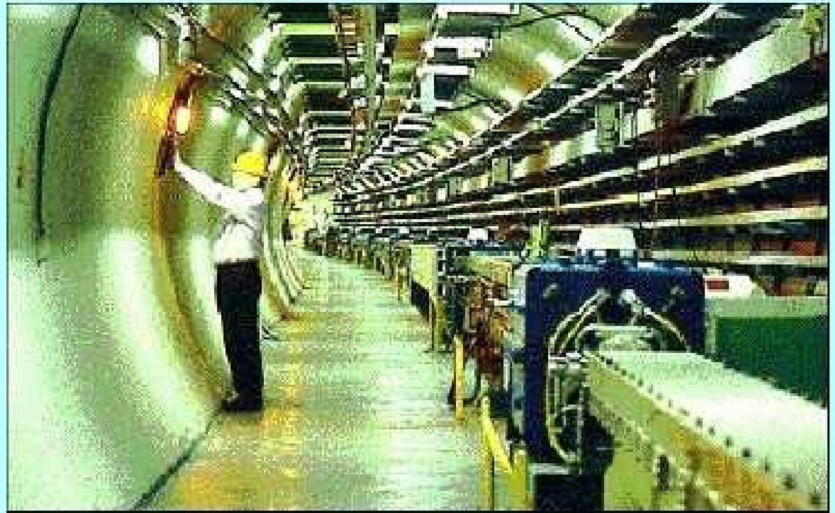
Electron synchrotrons are similar to proton synchrotrons except that the energy losses are greater.
